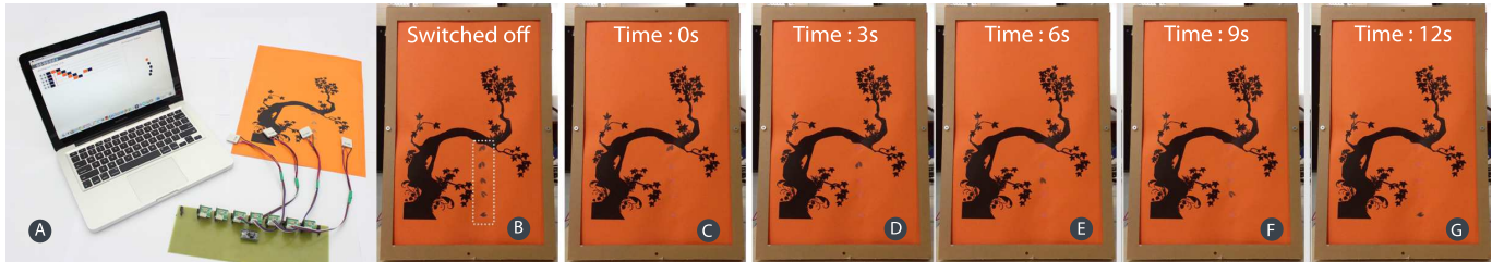
Figure 1. (a) The PaperPixels toolkit (b) Dotted circle shows the 5 animation frames of individual leaves appearing when the animation is switched off. (c) to (g) depicts animation of the painting every 3 seconds. PaperPixels Instructions Usage Video : http://goo.gl/zAeF30
